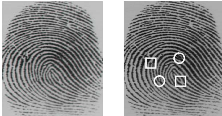
Suggestion #2: Extracted minutiae are indicated by different shapes (terminations with squares, bifurcations with circles)
